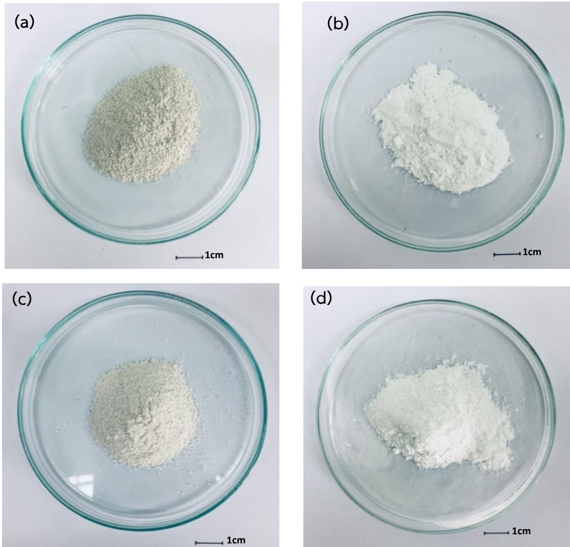
Figure 3 Unburned and burnt crushed seashells; Unburned crushed asiatic hard clam shells (a), Crushed asiatic hard clam shells are burned at 900^{\circ}\text{C} . (b), Unburned crushed semi-twisted ark shells (c) and Crushed semi-twisted ark shells are burned at 900^{\circ}\text{C} . (d)
